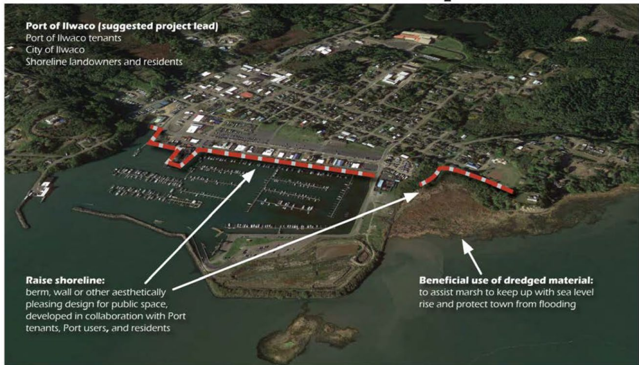
Figure 17. Ilwaco shoreline flood protection concept, developed by participants in the Bay to Bay project (Source: Blalock et. al. 2024).
