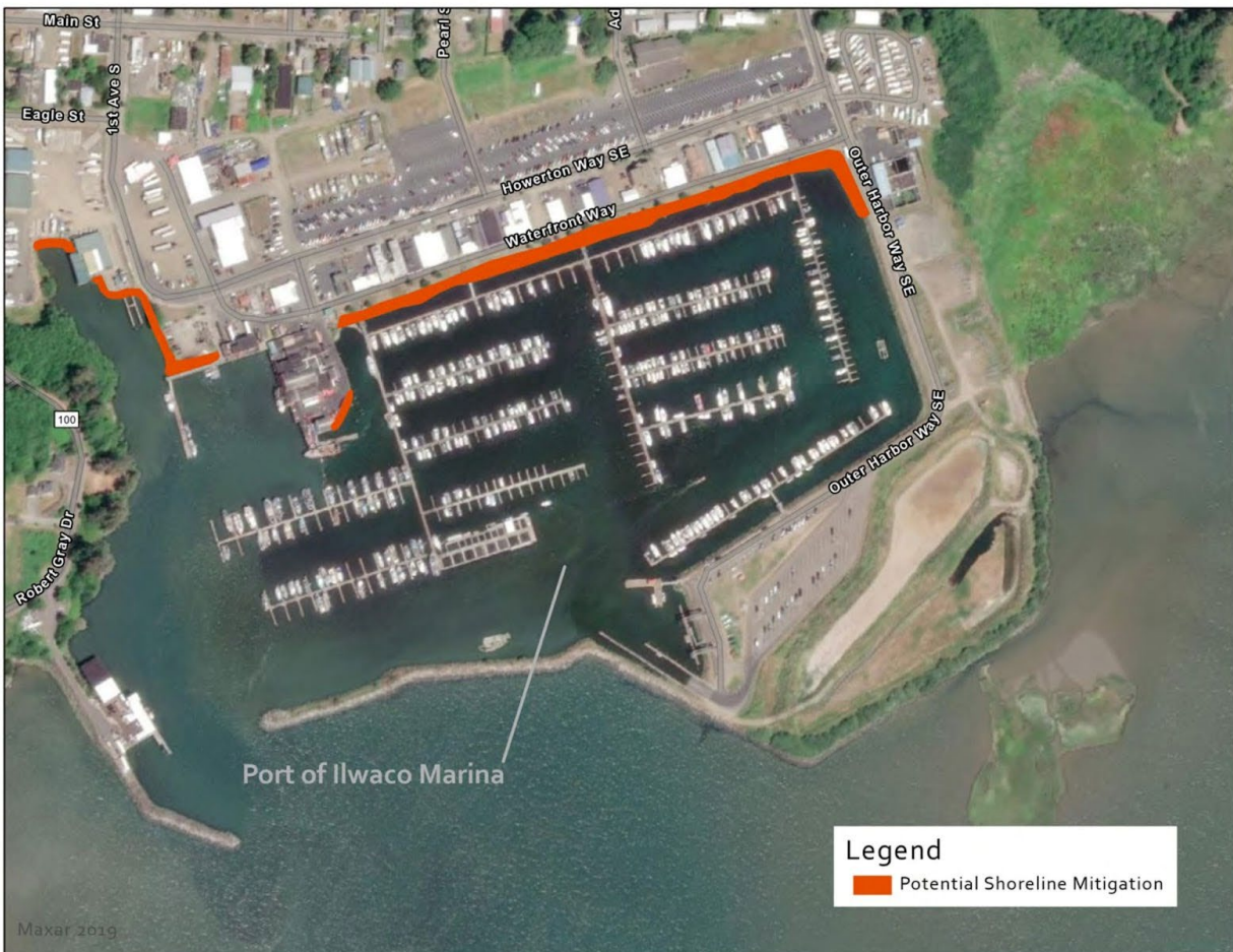
Figure 16. Conceptual drawing showing potential location of berm at Ilwaco Marina (Source: Moffat & Nichol)
